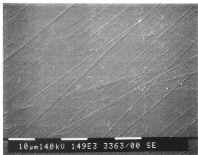
Figure 4 SEM of PPy-PTS membrane: plate side
